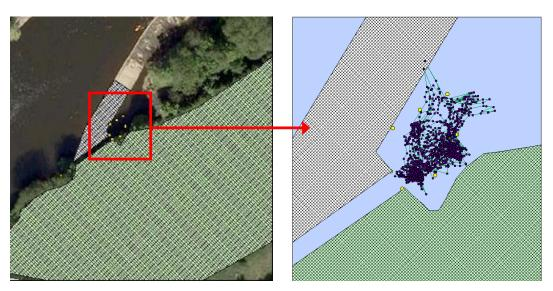
Figure 10. Digitised site layout (left) and an example fish track (right) plotted as polyline steps (green lines) between time stamped points (purple dots).
